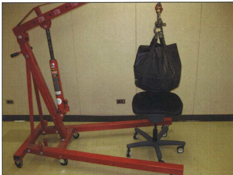
Figure 3 : Dynamic drop test set-up
