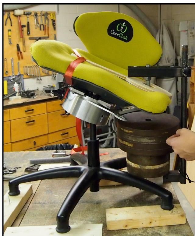
Figure 5: Lateral stability testing for the Core Chair.
